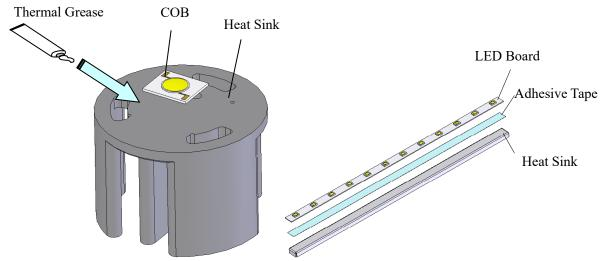
Connection with COB and the heat sink
