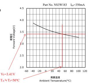
Figure 5. Calculation of T<sub>J</sub>
