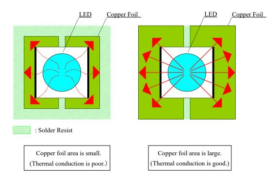
Figure 8. Copper foil pattern shape of the printed circuit board
