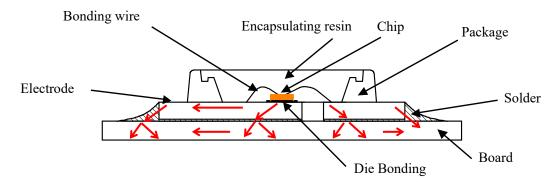
Figure 1. LED's structure and an example of the heat path (Example Part No. NS3W183)
