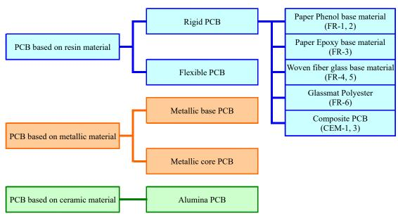
Figure 6. Classification of Printed Circuit Boards
