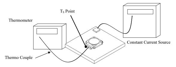
Figure 3. Thermal Measuring Set Up
