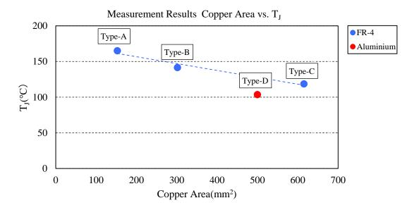
Figure 7. Thermal Measurement Results for Part No. NS6W183 (Copper area vs TJ)
